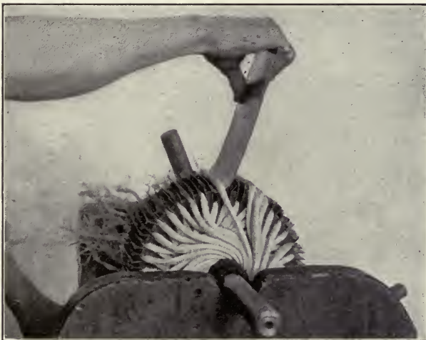
FIG. 68.—Inserting the last few top sides of coils. Note the shaping of the end connections of this winding alternately in and out to give the compact appearance shown in Fig. 71.
